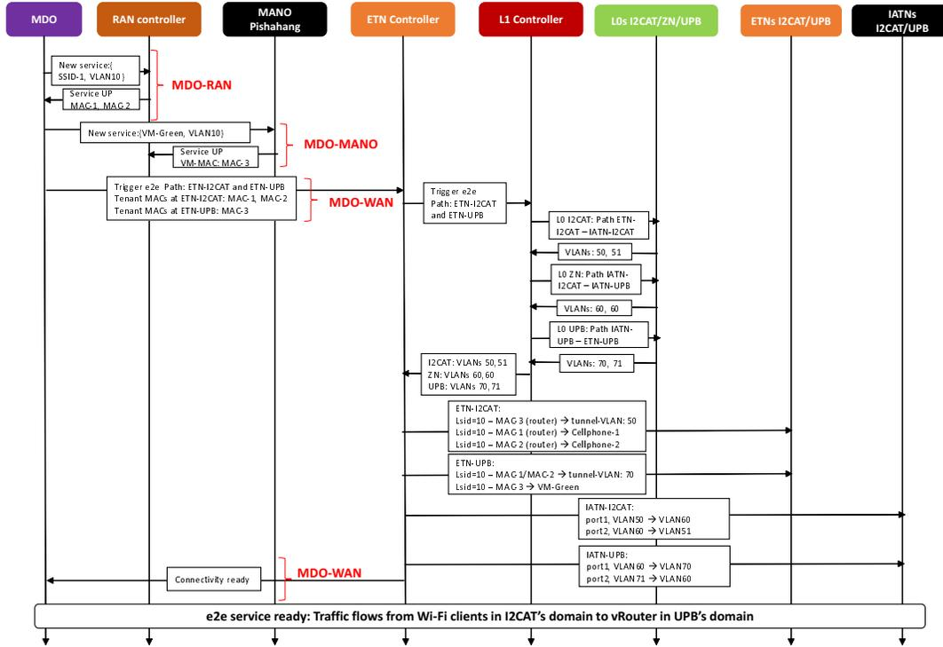
Fig. 4. Signalling involved in the provisioning of the e2e virtual Wi-Fi service
