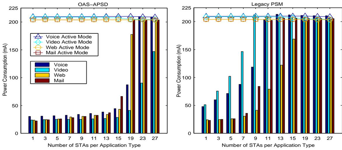
Fig. 8. Impact of the number of stations on the power consumption for *OAS-APSD* and *Legacy PSM*
