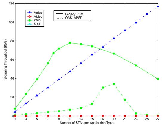
Fig. 10. Impact of the number of stations on the signaling load
