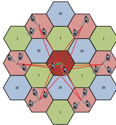
Figure 8: Frequency reuse patterns 3x1x1 used in simulations. The roman numerals depict the used frequencies.
